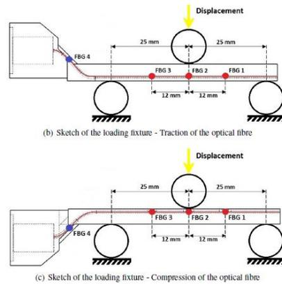
**Figure 1:** specimen test setup
