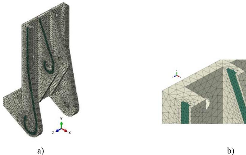
**Figure 3:** a) Rearward flap track support modelled with finite elements; b) detail of the component
