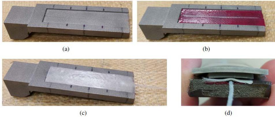
**Figure 2:** specimens produced with composite patch strategy to investigate the optical fibre embedment
