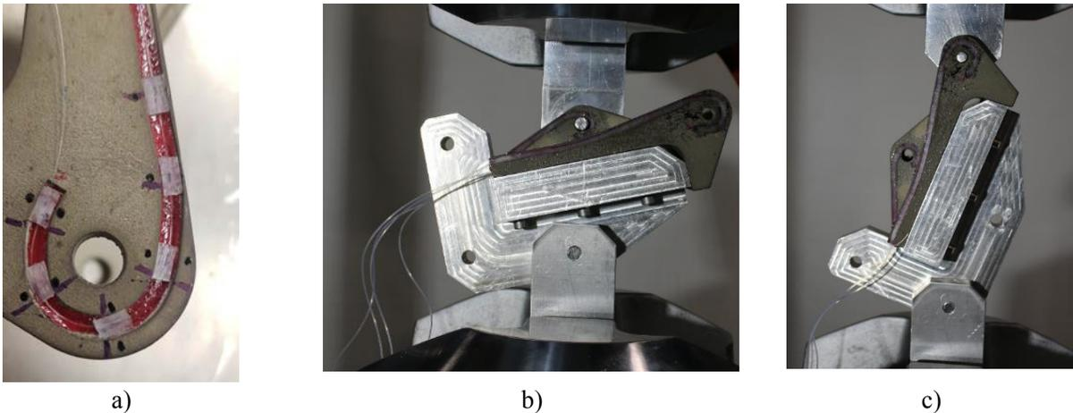
**Figure 6:** a) Composite patch version of the sensorized flap track rear support; b, c) flap track rear support subjected to testing
