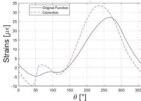
**Figure 5:** Example of original and corrected influence function
